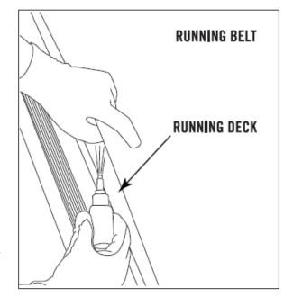
running deck. Tighten both rear roller bolts (matching up the marks for proper position) to original position. After you have applied lubricant, plug in the power cord, insert the safety key, start the treadmill and walk on the belt for two minutes to spread the lubricant.
