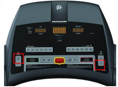
6) Press and hold the STOP key to exit Engineering Mode and return to normal operation.
